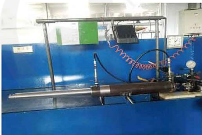
Cylinders final test
