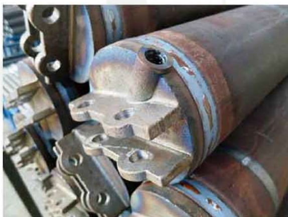
Threaded bushes welding
