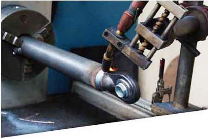
Bottoms and accessories welding on tubes
